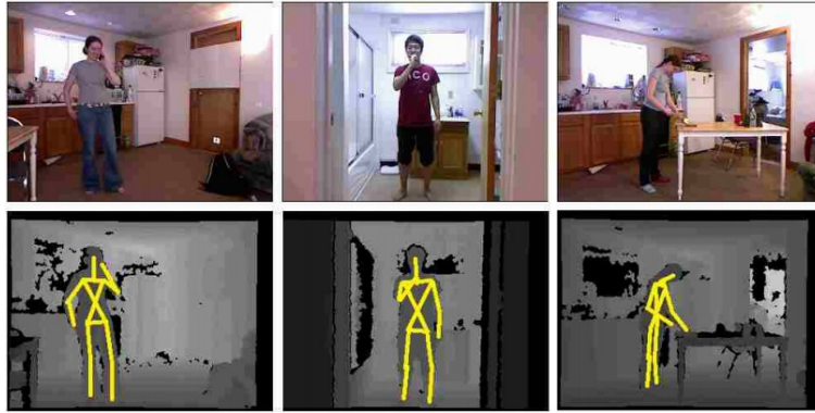
Fig. 2: Frames of human activities performed in a living environment extracted using an RGB-D sensor [23].
