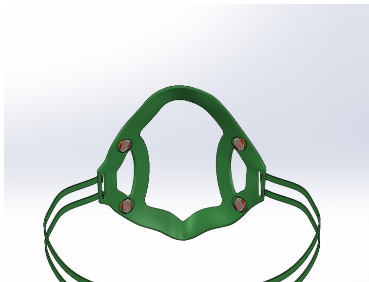
Figure 4. Mask brace with LDR sensors.
